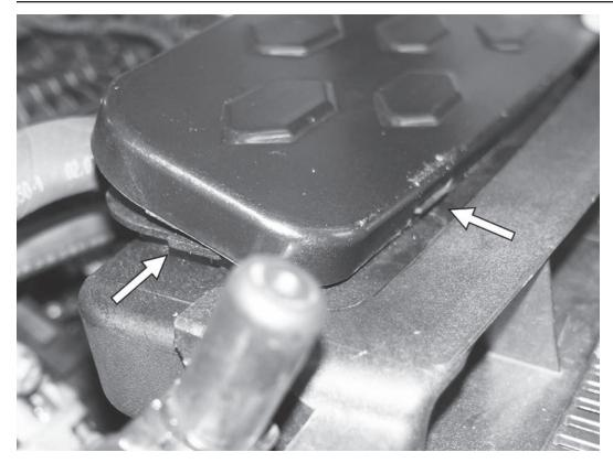
29) Install the airbox lid on the APR airbox by putting the front side of the cover on first. Ensure the two tabs on the front of the airbox go into the slots on the front of the airbox lid. Then, rotate the back of the airbox lid down. The lid will snap onto the tab on the right side of the APR airbox.
