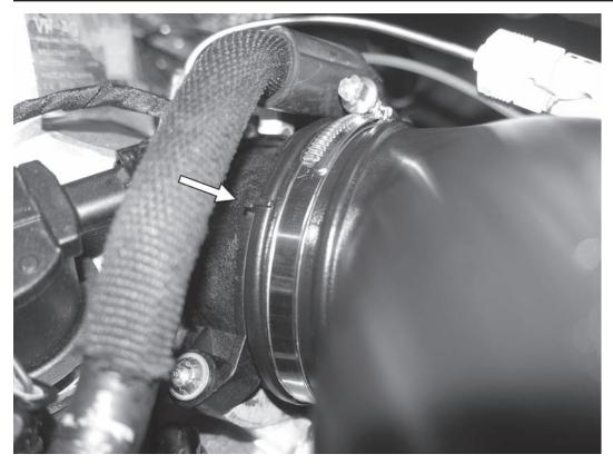
25) Loosely install the supplied hose clamps on both ends the APR inlet pipe. Install the APR inlet pipe on the APR turbo inlet adapter. The raised tab on the inlet pipe will align with the raised tab on the inlet adapter when correctly positioned.
