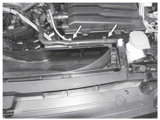
3) Remove the coolant line that runs over the airbox inlet scoop but lifting the coolant line out of the two retaining clips on the scoop.
