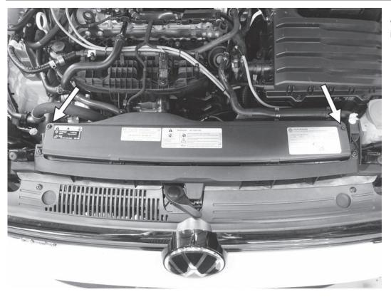
1) Raise the hood and remove the two T25 screws holding the airbox inlet cover.
