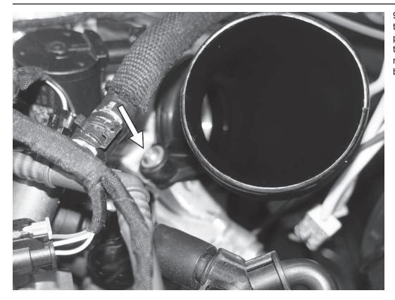
9) On the turbo inlet pipe, remove the T30 screw holding the inlet in place. Once removed, rotate the turbo inlet pipe clockwise, approximately 20°, to release it from the turbocharger.
