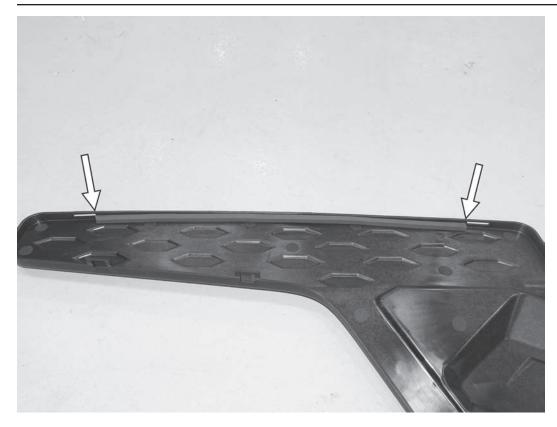
27) If installing the APR airbox lid, install the supplied foam tape on the bottom side of the airbox lid, between the two tab slots that are in the front of the lid.
