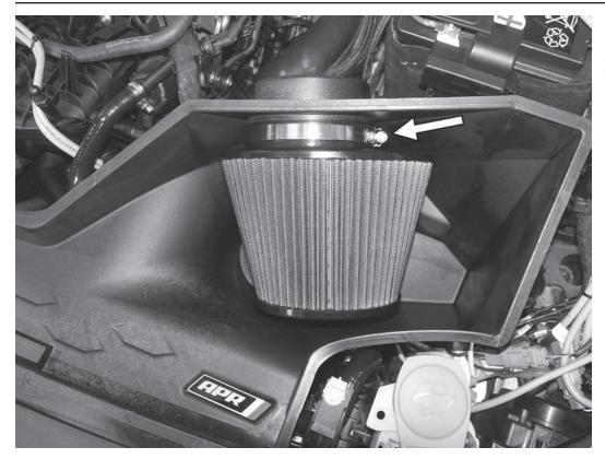
21) Install the APR filter with the supplied clamp onto the inside of the APR airbox. Make sure the filter is fully seated on the flange, and then tighten the clamp to 6Nm (53in-lbs).
