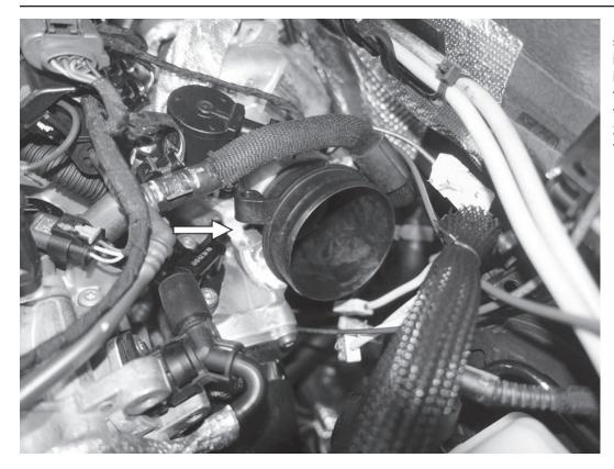
19) Lubricate and then install the supplied o-ring on the APR turbo inlet adapter. Push the inlet adapter into the turbo, ensuring the tab on the adapter seats into the slot on the turbo. The inlet adapter will be about 20° off clockwise from where it will finally sit.
