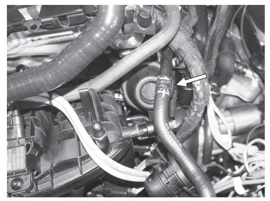
11) If not installing the APR coolant hose, skip to step 15. On the coolant line that ran over the airbox inlet scoop, remove the spring clamp that connects the hose to the metal pipe by the intake manifold. Remove the line from the pipe using a pick to loosen it. Use the supplied rubber cap over the metal pipe to keep the car from losing too much coolant.
