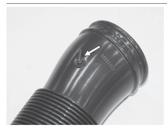
23) Install the supplied 90° barbed fitting into the rubber grommet in the APR inlet pipe.
