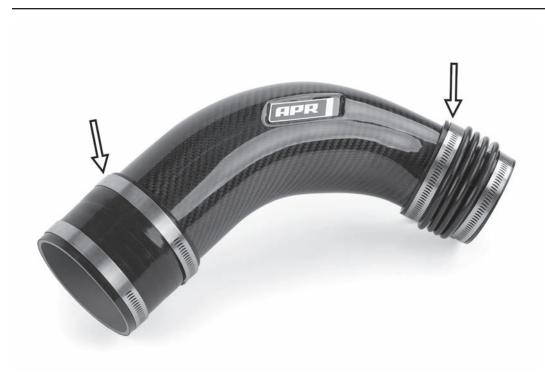
3) Loosely build the shown assembly with the four hose clamps, two couplers, and APR inlet tube. After peeling off the adhesive backing, attach the APR logo in the indented location on the inlet tube.
