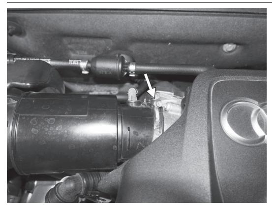
1) Raise the hood on the car, and then loosen the hose clamp on the back side of the accordian intake tube at the throttle body.
